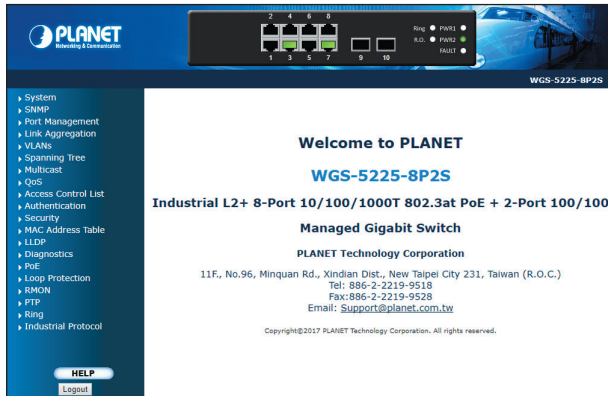
Figure 5-3: Web Main Screen of Wall-mount Managed Switch
